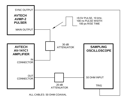
The recommended test set-up is shown above.
